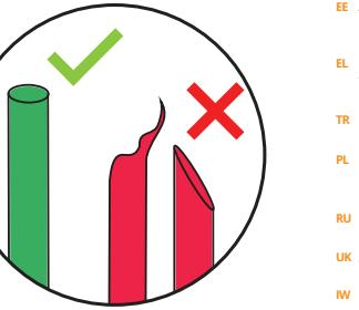
**EN** Ensure the filament is cut correctly before inserting into the pen.
